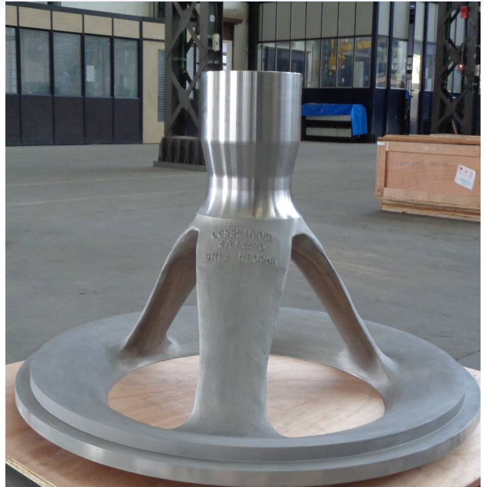
Hub in Duplex Grade for Centrifuge Equipment
