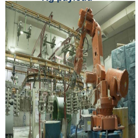
Automated back up coting with Robot of 210 Kg payload
